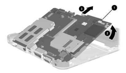
Removing the System Board
